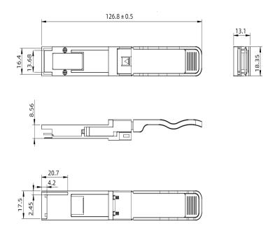
Unmarked Dimensional Tolerance ±0.2mm, units: millimeters
