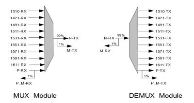
Note: The above figure is the wiring diagram of MT2010-CWDM-MUX8-4761-MPG-00 product
