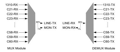
Note: The above figure is the wiring diagram of MT2010-DWDM-MUX40-CH21-CH60-MG-00.
